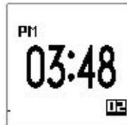
**NOTE:** The watch will automatically set the time according to GPS satellites. However, you must set the correct Time Format, Time Zone and Time Mode by navigating the MENU Screen.
